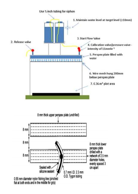
Figure 3.1. Principal components of the rainfall simulator (top) and of Perspex plate (bottom)
