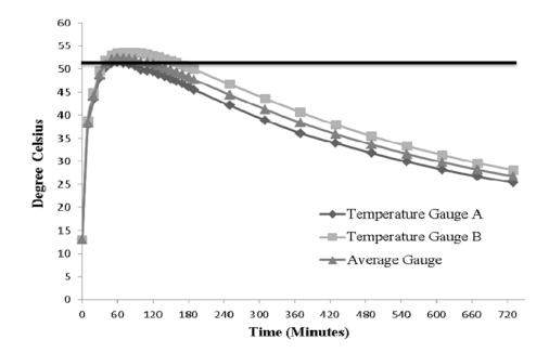
**Figure 4.5.** Temperature vs. time over 12 hr. Horizontal bar indicates 52°C, which is the temperature guideline (Fehily, Timoney and Company, 1999)
