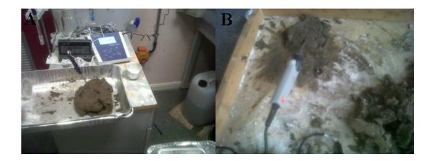
Figure 4.2. The experimental setup for the preliminary test. A) – temperature monitoring of 2 kg sludge cake and B) – a temperature probe close up.
