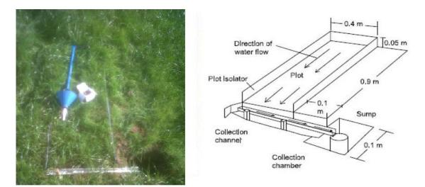
**Figure 5.2.** Picture of micro-plot fitted with runoff off collection channel and micro-plot set up.
