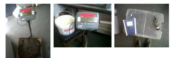
Figure 4.3. The measurement of lime and sludge, and sealed container mixture with temperature probes inserted.
