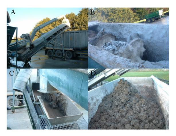
**Figure 4.6.** A) Standard lime-sludge mixing apparatus at a WWTP, B) Pugmill Augers, C) completion of sludge and lime mixture on transfer belt, D) truck collection.
