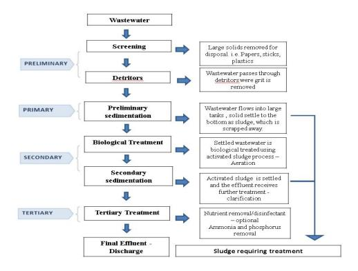
Figure 2.2. Illustration of a simplified wastewater treatment process (adapted from Antille et al., 2011; Metcalf et al., 2003).
