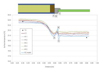
Fig. 15. Temperature distribution for Specimen 4 with PVC frame window.
