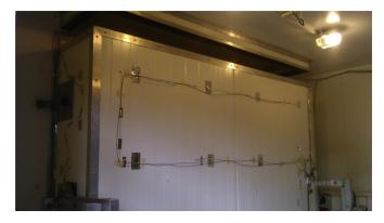
Fig. 3. Metering box fastened to the surround panel.
