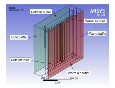
Fig. 9. The 3D view of Specimen 1 with surrounding elements. (For interpretation of the references to color in this figure, the reader is referred to the web version of this article.)
