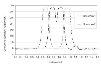
Fig. 8. Indoor convective coefficients.
