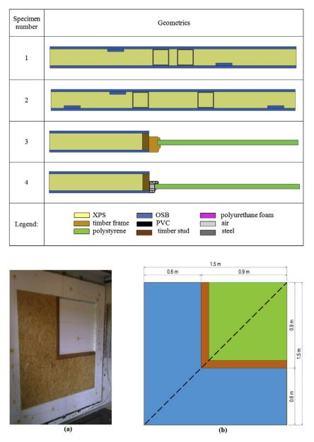
Fig. 2. Specimen 3 mounted into the hot box surround panel (a) and Specimen dimensions (b).
