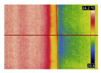
Fig. 5. IR image of Specimen 3 with a timber frame window.
