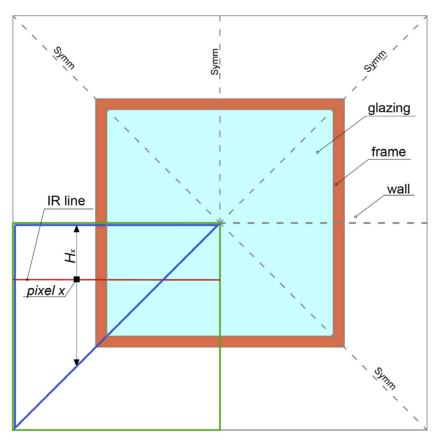
Fig. 6. Geometry of a window installed into a wall. Tested section outlined in green, section for calculation outlined in blue. (For interpretation of the references to color in this figure legend, the reader is referred to the web version of this article.)
