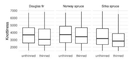
**Fig. 1** Board knottiness value according to X-ray measurement by species and thinning regime
