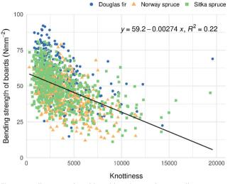
Fig. 2 Bending strength and board knottiness value according to X-ray measurement
