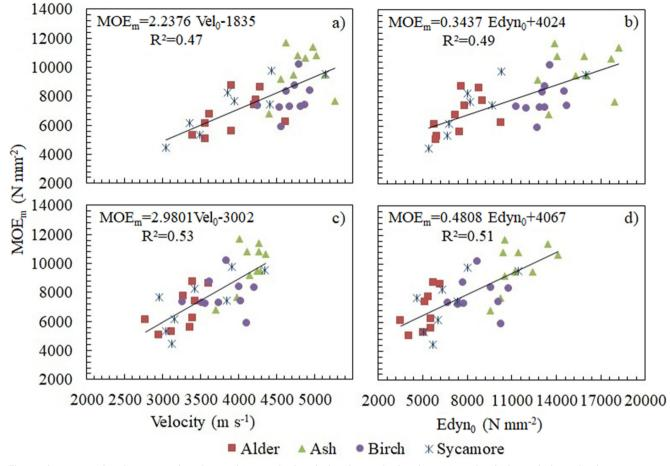
Fig. 4 Linear regressions between static MOE<sub>m</sub> and (a) TreeSonic velocity, (b) TreeSonic Edyn<sub>0</sub>, (c) MTG velocity, and (d) MTG Edyn<sub>0</sub>
