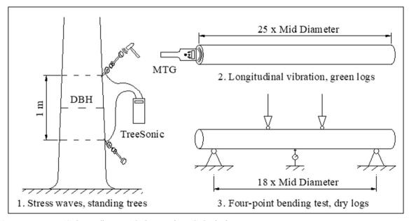
Fig. 1 Measurement set up. (1) On standing trees. (2) On green logs. (3) On dry logs
