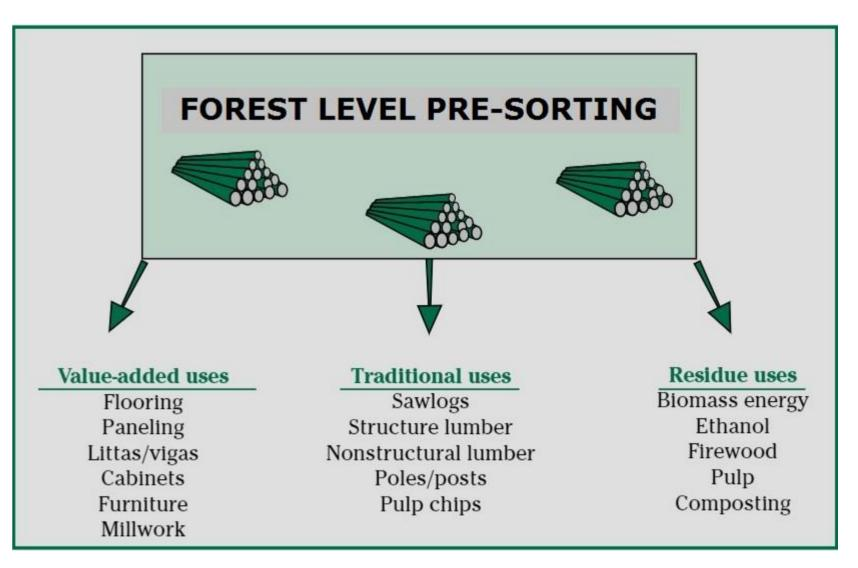
Fig. 3 : Hierarchy of uses for small-diameter material
