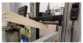
Figure 5: Failure behaviour of DLT member (DLT - 2)
