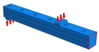
Figure 7: Numerical model geometry subjected to four-point bending utilising half symmetry (DLT-D20-S100).
