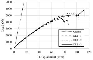
Figure 4: Load-displacement behaviour of the DLT members
