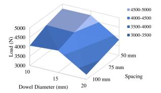
*Figure 13.* The influence of dowel diameter and dowel spacing on maximum load ( $F_{max}$ ).
