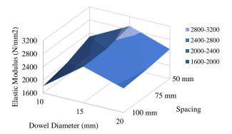
*Figure 14.* The influence of dowel diameter and dowel spacing on elastic modulus.
