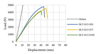
Figure 11. Numerical load-displacement curves for specimens with 15 mm diameter dowels (D-15 Series).
