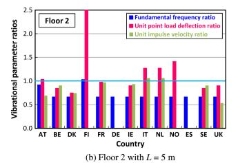
**Fig. 10.** Vibrational parameter ratios for Floors 1 and 2.
