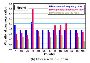
Fig. 14. Vibrational parameter ratios for Posi joist floors.
