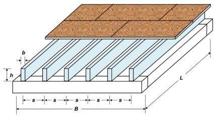
Fig. 9. A typical floor constructed with solid timber joists.
